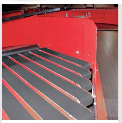
The compact Full Belt Merge (FBM) operating at conveyor speeds up to 2 m/s, is an alternative to Strip Belt Merge (SBM). Designed for flawless and repeatable merge function where a closed belt carrier is preferred. Automatic belt tracking is included as a standard feature.
