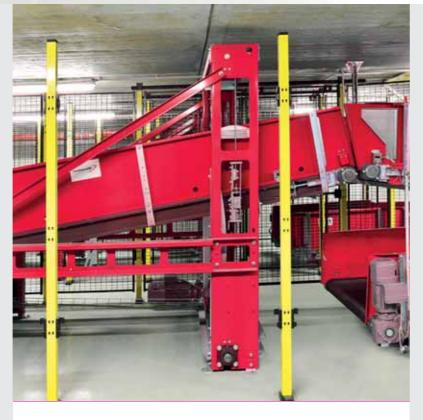
The motion06 High Speed Diverter (HSD) is available at various performance levels, capable of reaching a capacity of 2,700 items/ hour. Due to a newly developed drive concept (Class IE4), the m06 Diverter is highly energy efficient and its the flexible design of the construction makes the changing of the swivel direction a simple
