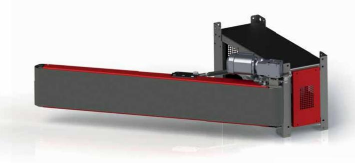
Vertical Diverters are used wherever special pieces of baggage need to be discharged from the main flow of baggage. Speed, strength and resilience become the key features for such an application, and m06's Vertical Sorting Unit (VSU) offers precisely that and more. With a capacity of up to 2,000 pieces of baggage per hour, the lifting mechanism comes with two steel-reinforced tooth belts that lifts and lowers the belt conveyor deftly.
